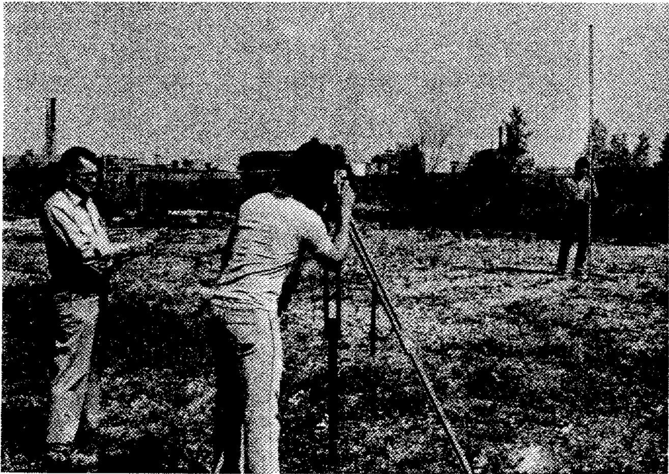
Figure 3. Typical survey party. Instrument man sets up instrument, reads intercepts of instrument wires through telescope focused on rod. Rodman holds rod erect on monument or turning point, verifies rod is vertical by observing rod level. Field Recorder makes entries in book, calculates foresights and backsights from three readings, verifies all are correct. Usually recorder is field engineer in charge of party—his duties also include route planning and selection of instrument sites so that foresights and backsights are approximately equidistant and provide optimum view of all monuments available to instrument man at this location.
